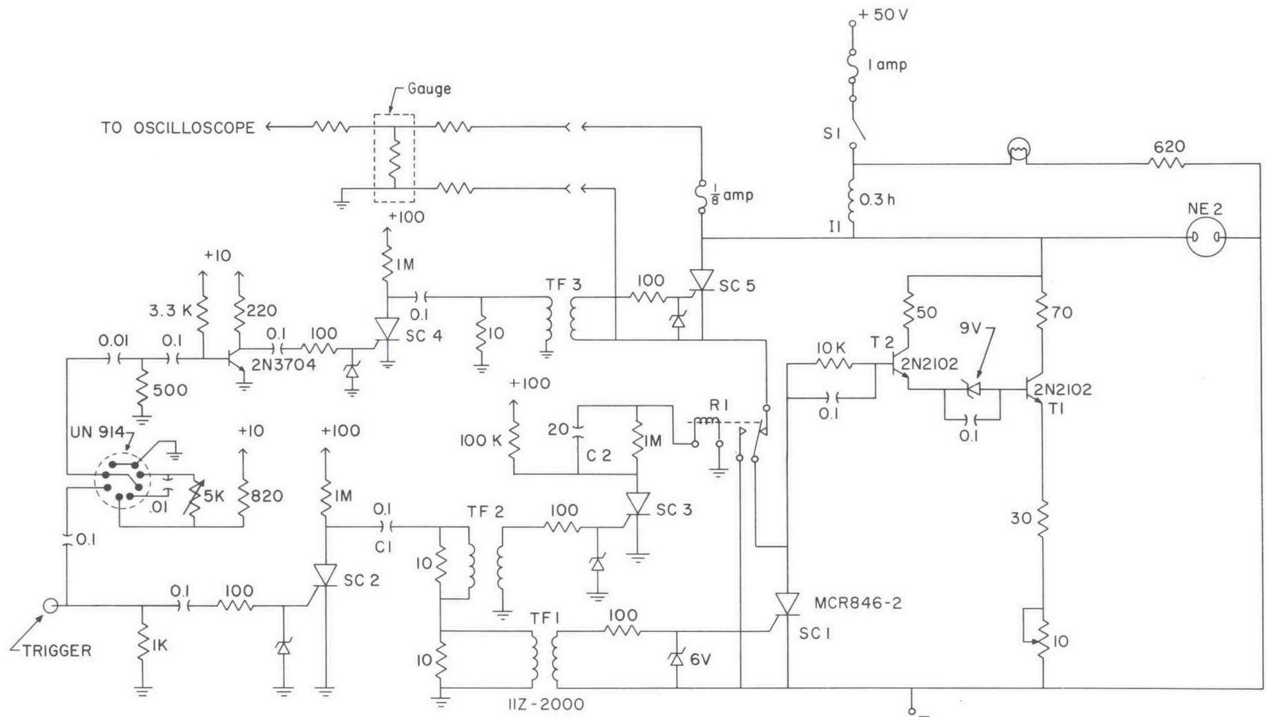
Fig. 22. Schematic of manganin gauge constant current supply.
